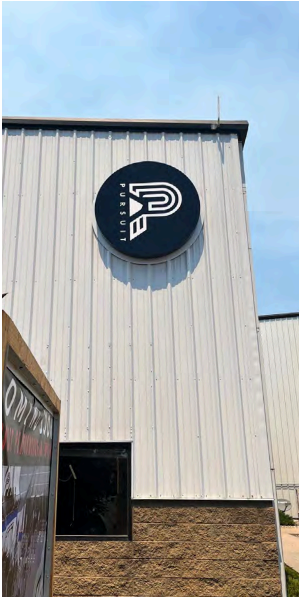
5' diameter, round wall cabinet with reverse pan channel illuminated logo and halo illumination.
