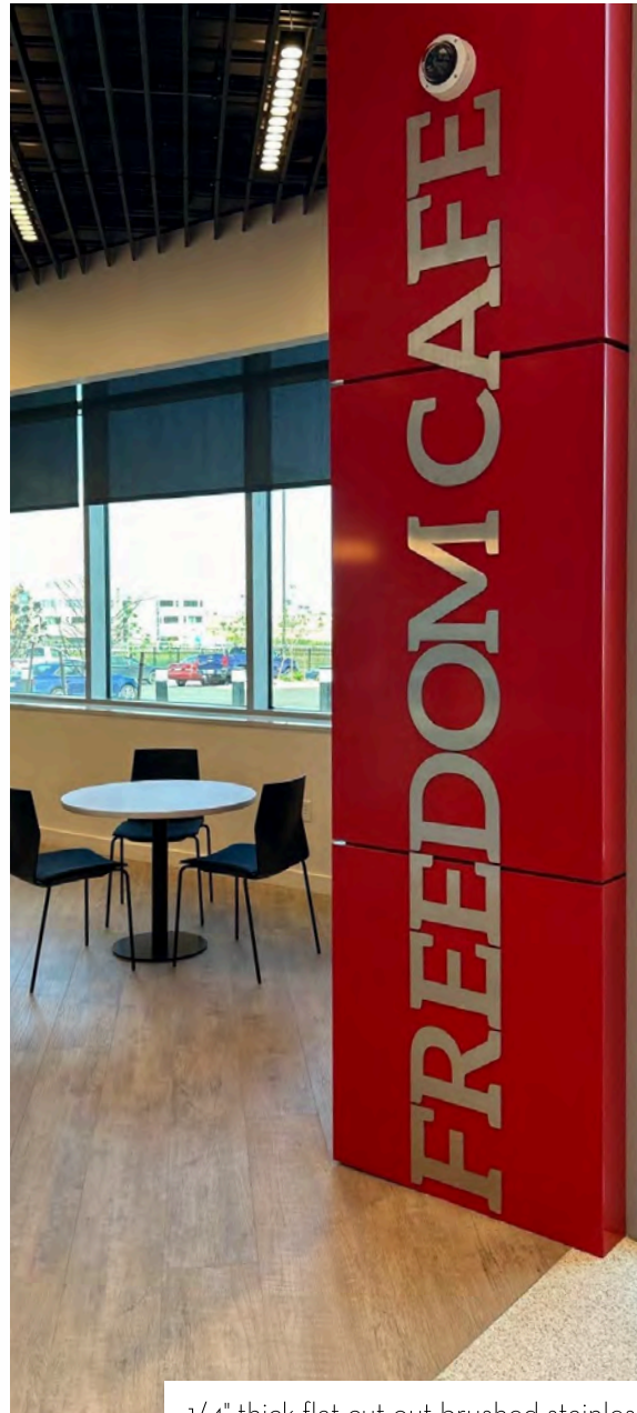
1/4" thick flat cut out brushed stainless steel flat cut out letters.
