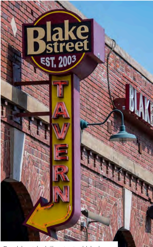
Double-sided illuminated blade sign with open face neon channel letters.
