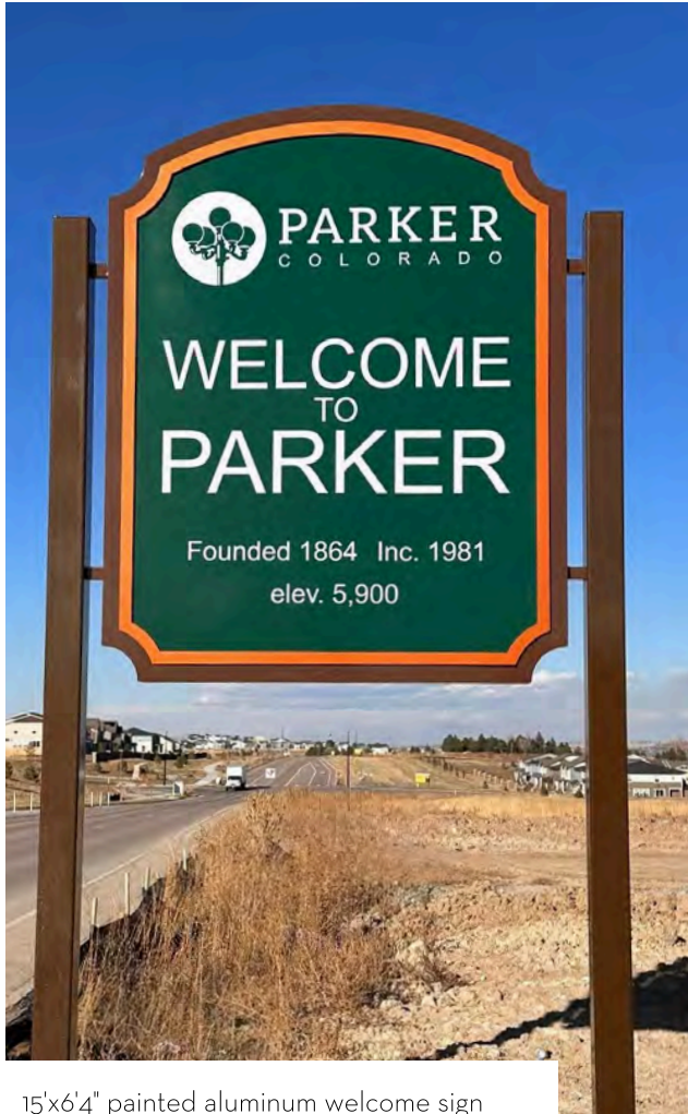
15'x6'4" painted aluminum welcome sign with reflective film graphics.
