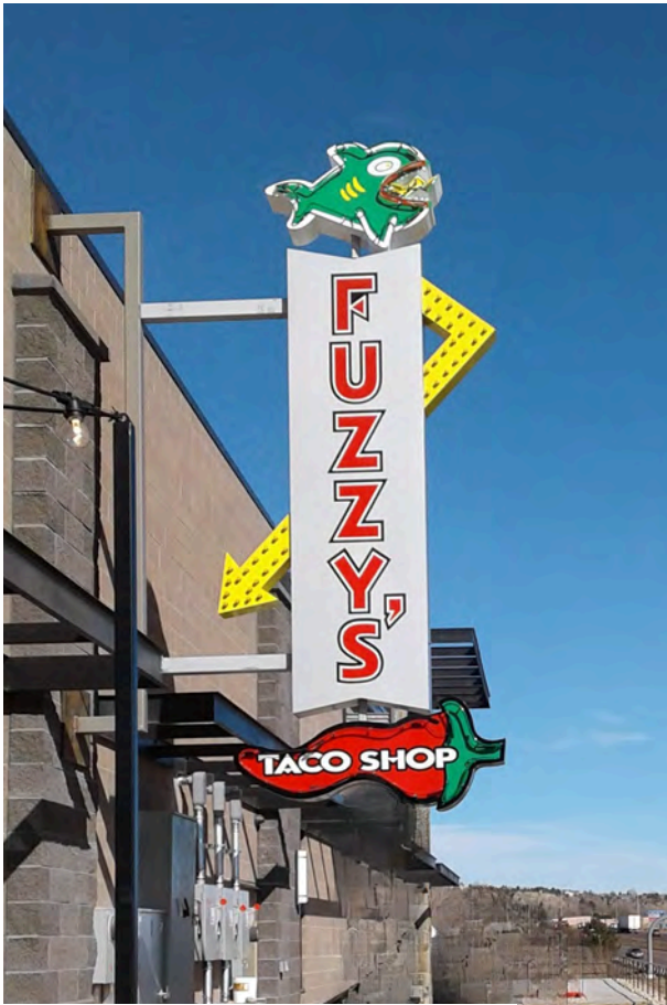
Double-faced 10' painted aluminum cabinet with film graphics. Yellow arrow features exposed bulbs.
